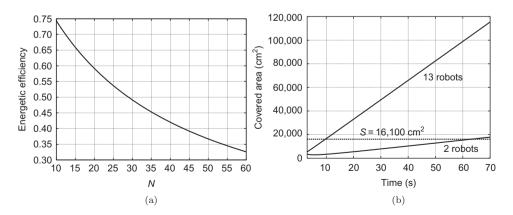
Figure 3. (a) Energetic efficiency of the 'Jasmine' swarm for Equation (6) at a constant swarm density; (b) plot of covering rate from Equation (14).
