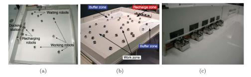
Figure 6. (a) Experimental set-up for the small arena; (b) experimental set-up for the large arena; and (c) docking station with IR slots, allowing an 'energy-smelling' approach.
