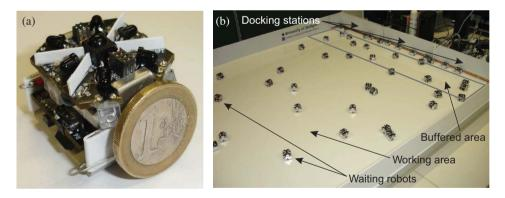
Figure 1. (a) The 'Jasmine III' micro-robot; (b) Collective energy foraging in a swarm of 50 'Jasmine' micro-robots, showing docking stations, recharging robots and robots waiting near the docking station.
