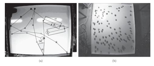
Figure 4. Coverage by (a) 2 and (b) 13 robots. Ten seconds of motion (10 images) are shown, as difference images extracted from the video sequences.
