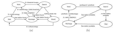
Figure 5. Behavioural model for (a) spontaneous and (b) inertial robots.
